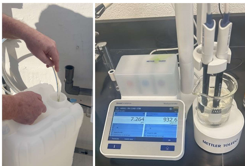
Figure 5. Picture of sample collection and analytical equipment used to analyze for pH and Salinity.
